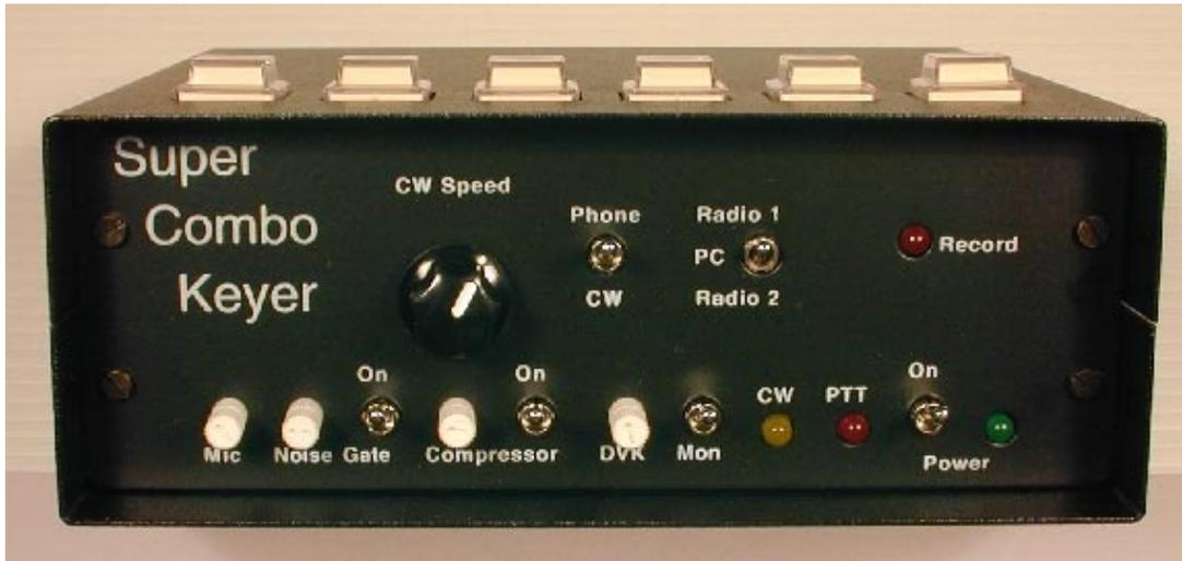
The unit's front panel contains all the controls used during normal operations, and several controls used only during initial configuration. The figure shows the location of all front panel controls. Details about their use can be found in the relevant sections of Chapter 4.
