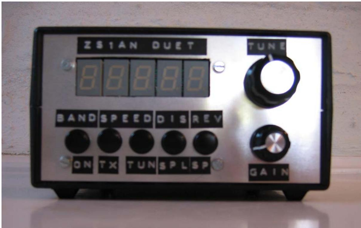
Figure 7 - Front Panel Layout
