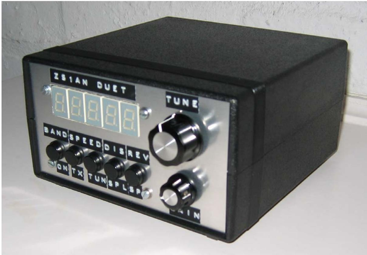
Figure 1 – The “Duet” Dual-Band CW Transceiver
