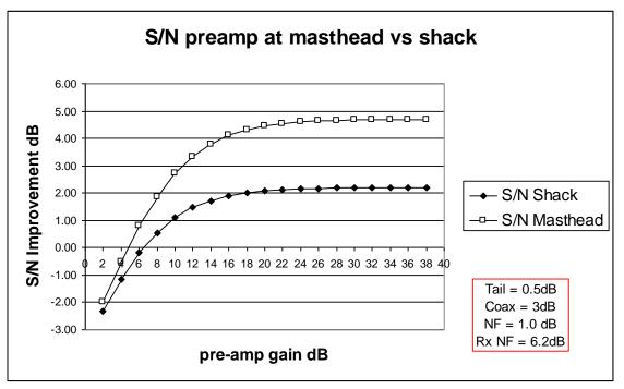
Fig 1: Because the coax loss before the pre-amp has a large effect on the overall Noise Figure, it is better to keep it to a minimum by placing the pre-amp close to the antenna.
