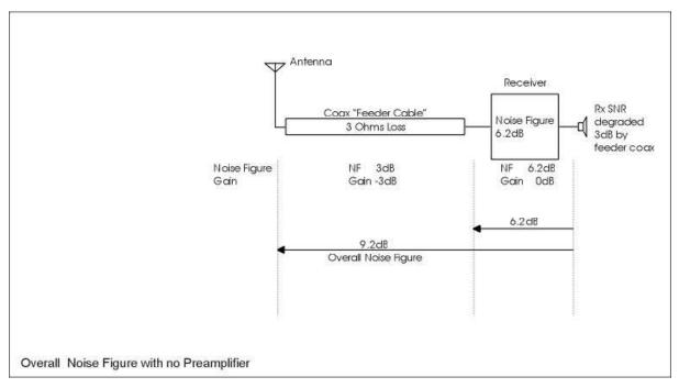
In this example, adding a good 20dB pre amplifier with a 1dB Noise Figure improves the overall Noise Figure from 9.2dB to 1.75dB and the S/N ratio by 7.45dB. The 3dB degradation from the feeder loss becomes a 4.45dB enhancement due to the gain and improved Noise Figure.
