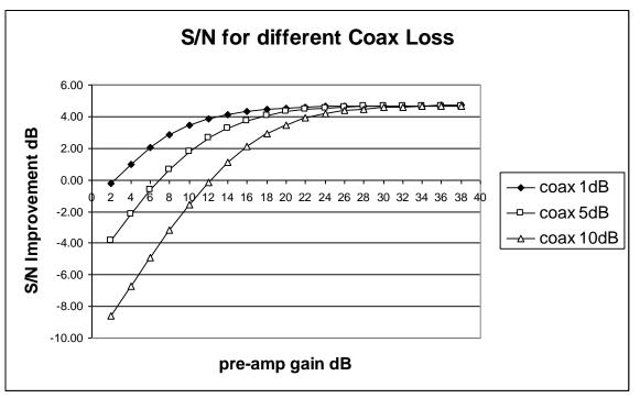
Fig 3: Coax loss after the pre-amp can be made up with pre-amp gain. Increasing pre-amp gain past a certain point has little effect on the overall Signal to Noise improvement, but will reduce the receiver's dynamic range and can add intermodulation distortion in the presence of strong signals.
