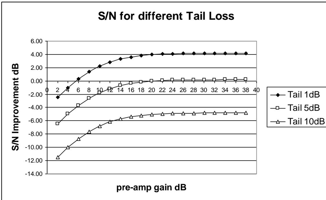
Fig 4: Coax loss before the pre-amp adds directly to the overall Noise Figure and should be kept as low as possible. Too much loss before the pre-amp will result in no Signal to Noise ratio improvement or a degraded Signal to Noise ratio, no matter how much gain the amplifier has.
