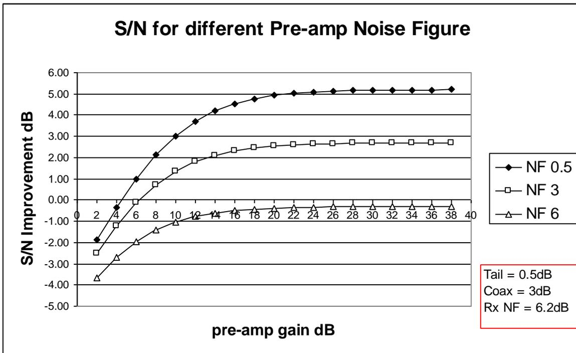
Fig 2: If the pre-amp or overall Noise Figure is poor, no amount of gain will result in an improved Signal to Noise ratio.
