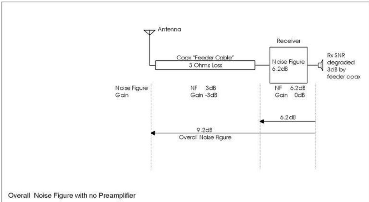
In this example, adding a good 20dB pre amplifier with a 1dB Noise Figure improves the overall Noise Figure from 9.2dB to 1.75dB and the S/N ratio by 7.45dB. The 3dB degradation from the feeder loss becomes a 4.45dB enhancement due to the gain and improved Noise Figure.
