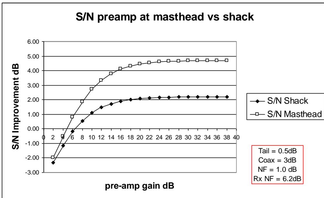
Fig 1: Because the coax loss before the pre-amp has a large effect on the overall Noise Figure, it is better to keep it to a minimum by placing the pre-amp close to the antenna.
