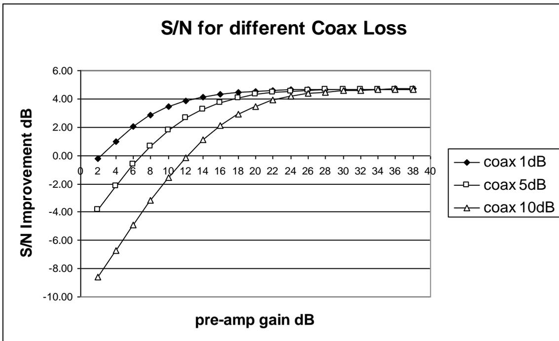
Fig 3: Coax loss after the pre-amp can be made up with pre-amp gain. Increasing pre-amp gain past a certain point has little effect on the overall Signal to Noise improvement, but will reduce the receiver's dynamic range and can add intermodulation distortion in the presence of strong signals.
