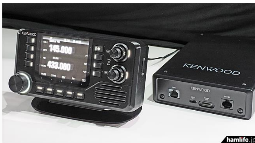
JVC- KENWOOD exhibited a car transceiver under development. It consists of a large control unit (controller) and the radio body
