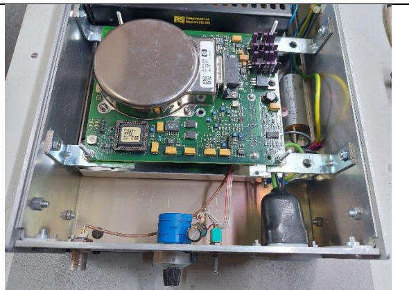
HP E1938A 'Hockey puck' oscillator as used in the HP Z3815A GPS disciplined 10MHz frequency standard
