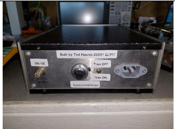
Rear of unit showing vernier frequency trim control.
