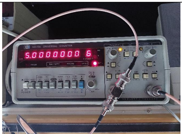
This shows a frequency count from the Hockey Puck unit obtained using a gate from the 1pps square wave output from the Z3815A GPS disciplined oscillator
