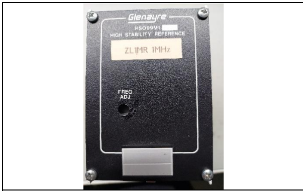
1MHz frequency standard ex an old Telecom system. Calibrated against the GPS 10MHz oscillator
