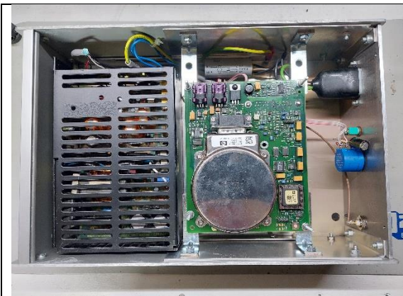
Top view of 10Mhz unit. Power supply on left oscillator on the right, rear view of blue vernier trim resistor
