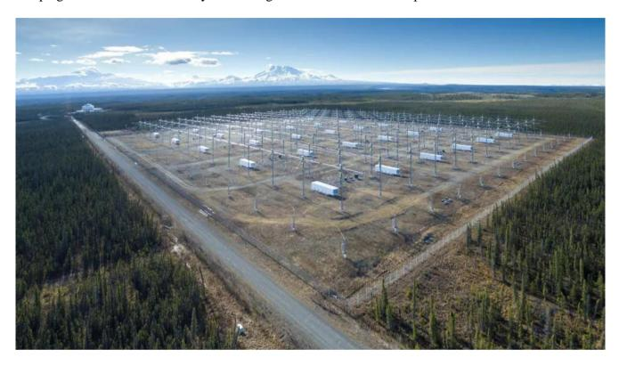
HAARP consists of 180 antennas designed to transmit signals into the ionosphere, which stretches from 30 miles (48 kilometers) to 600 miles (965 km) above sea level and is seen as the area where Earth's atmosphere meets space, according to NASA. The ionosphere plays an important role in radio transmission, as it reflects radio waves. Many satellites occupy this region of the atmosphere, which is heavily influenced by solar weather.
