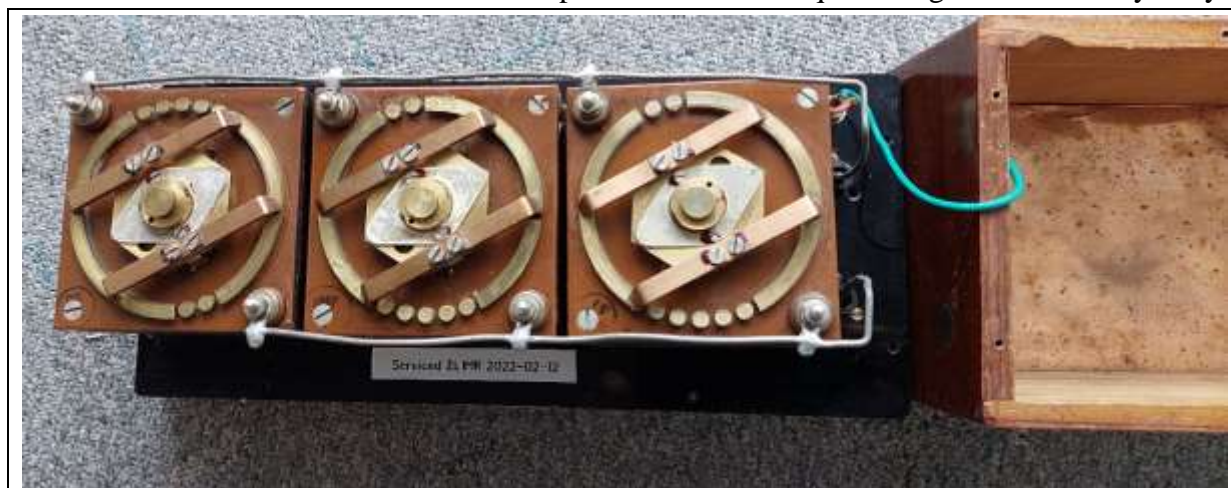
Condenser Decade Box – contact wipers and copper shielding inside box
