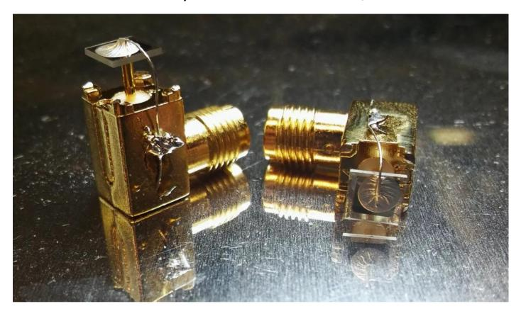
Radioactive diamond batteries were first developed by a team of physicists and chemists from the Cabot Institute for the Environment of the University of Bristol. The invention was presented as a betavoltaic device, which means that it's powered by the beta decay of nuclear waste.
