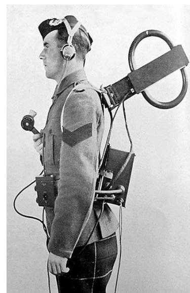
Right Image is Infantry walkies for the purpose of close radio communication with tanks, year 1936 Power 0.3 W, frequency range 51-64 MHz 6m Mag Loop for portable operation...1936
