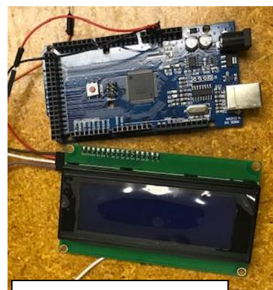
Ian ZL1AOX Mega2560 Arduino with K3NG Software
