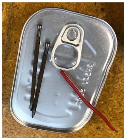
Jackie ZL1WA used 2 nails for her keyer, whilst John ZL1BYZ used the tab on a sardine can for his key
