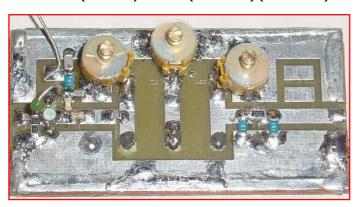
This PCB (left) is used to drive the 648 to 1296 MHz Multiplier, and is fitted with an additional 5 dB attenuator to drop the + 12 dBm output to + 7 dBm. It also gives a broadband termination to the following multiplier enhancing stability.
