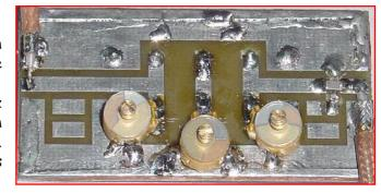
The filter I am building is to be used in a 1296 MHz beacon. This particular filter was to be tuned to 648 MHz before building the multiplier section on board. The filter has 2.1 db loss, (including cable loss) rejection @ 324 MHz -55 dB, 216 MHz -60 dB, 108 MHz -70 dB.
