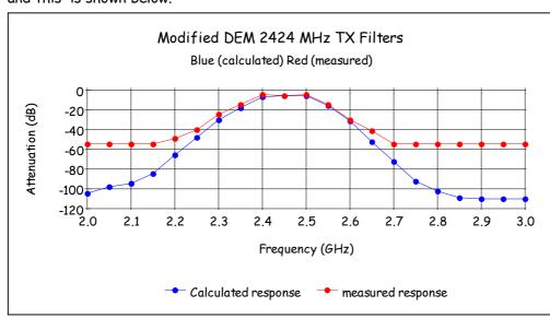
The red trace was only made down to -55 dB, this being the noise floor of the setup. Filter rejection continues further. Ripple appears in the top of the filter which I think is due to the interaction of the filters at their common point. The MMIC amp will be replaced at that point and I expect the ripple to reduce. Filter rejection of the LO at 2280 MHz improved from ~ 5dB to ~25 dB (30 dB filter loss @2280 MHz - 5 dB filter
