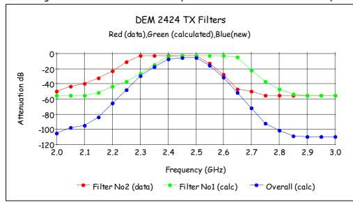
I carefully measured the dimension of the hairpin stripline along its centre line carefully with a pair of digital calipers. The 1st filter was to be moved from it's centre frequency of 2300 MHz to 2500 MHz or be shortened by a factor of 0.92. This equates to ~ 3.6mm off the filter length or 1.8mm off each each open end of the hairpin.
