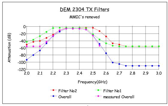
The frequency plot adjacent shows the filter response of both the  $1^{st}$  and TX hairpin filters. The 1st filter after the mixer, Filter No 1, (green) ( ~ 2.2 - 2.4 GHz) passes wanted (2424 MHz) and the LO (2280 MHz) with minimal attenuation. With both these signals present in following MMIC amp there will be added intermod, generating
