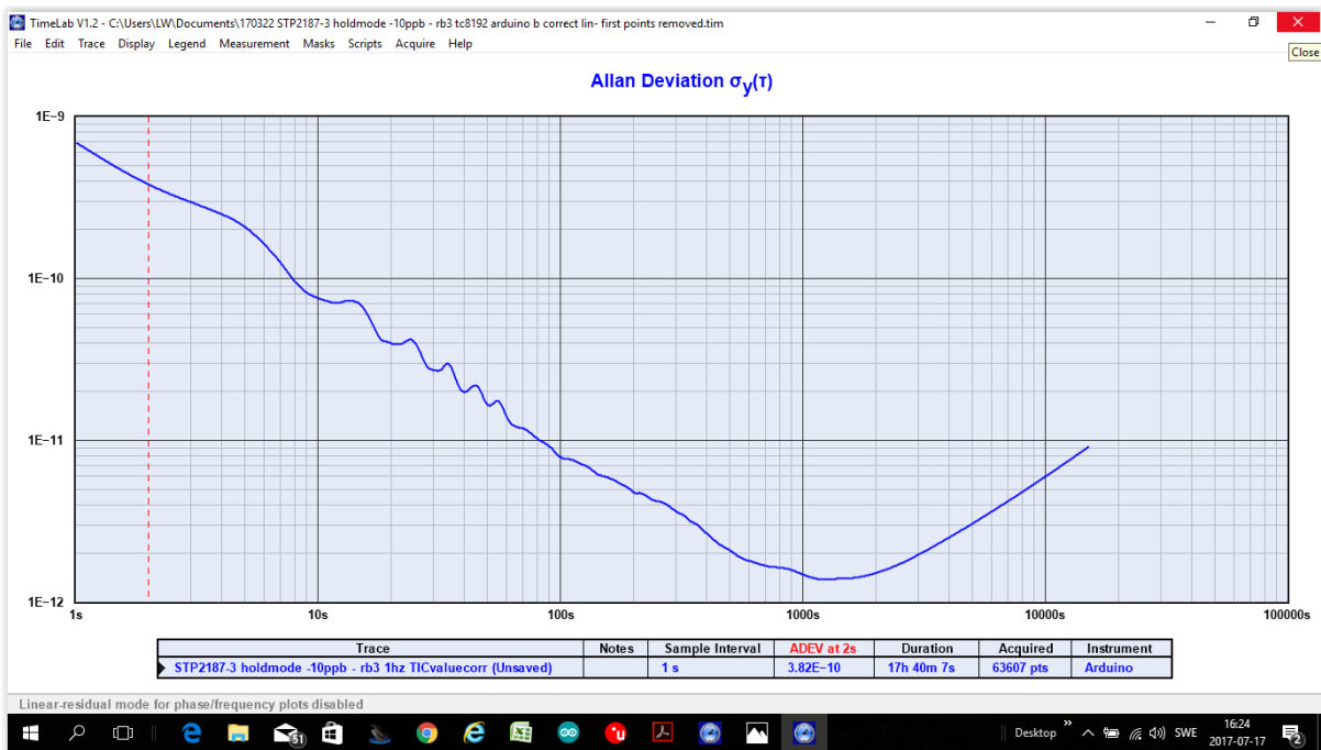
Figure 9. OCXO in holdmode measured with Arduino TIC (OCXO offset about 10ppb)
