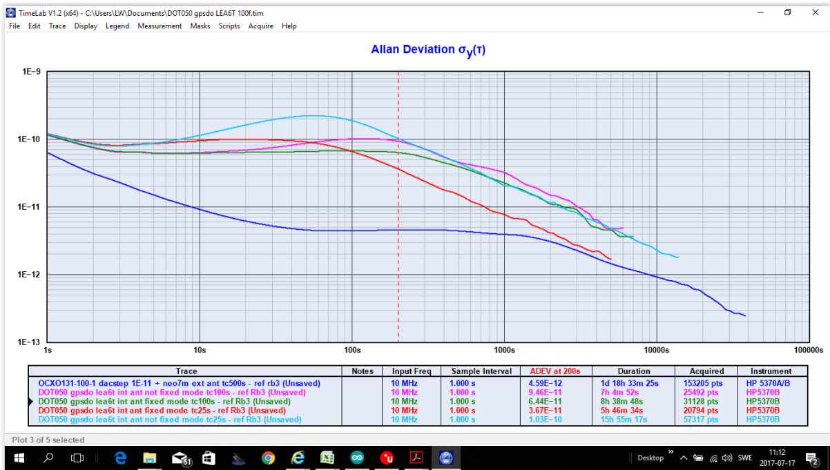
Figure 8. ADEV's of two of my GPSDO's. DOT050 is a VCTCXO, here tested with different GPS modes and time constants.
