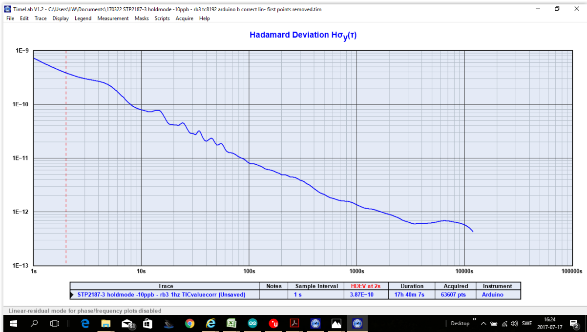
Figure 10. OCXO in holdmode measured with Arduino TIC
