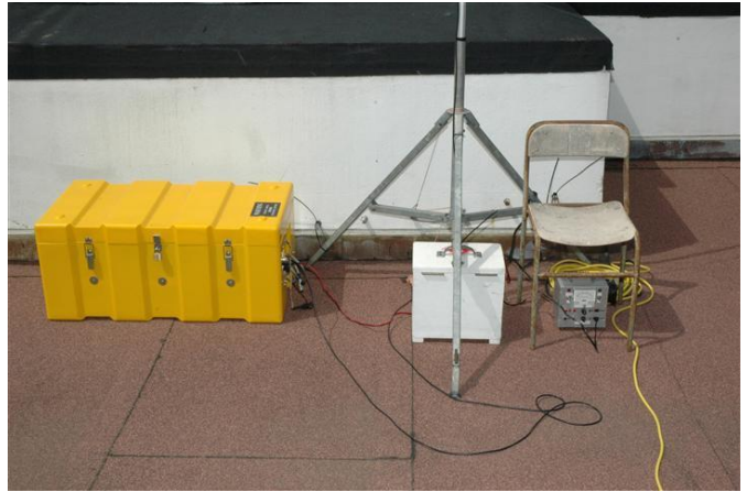
The repeater battery box, stand and battery charger.
