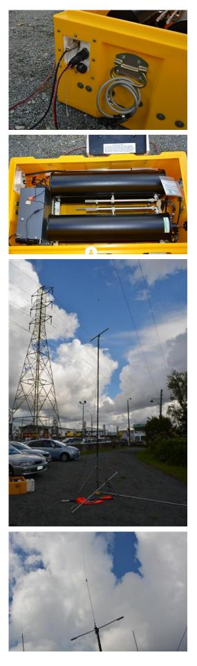
The power and antenna inputs to the Repeater. Always have the antenna connected before the power is connected.
