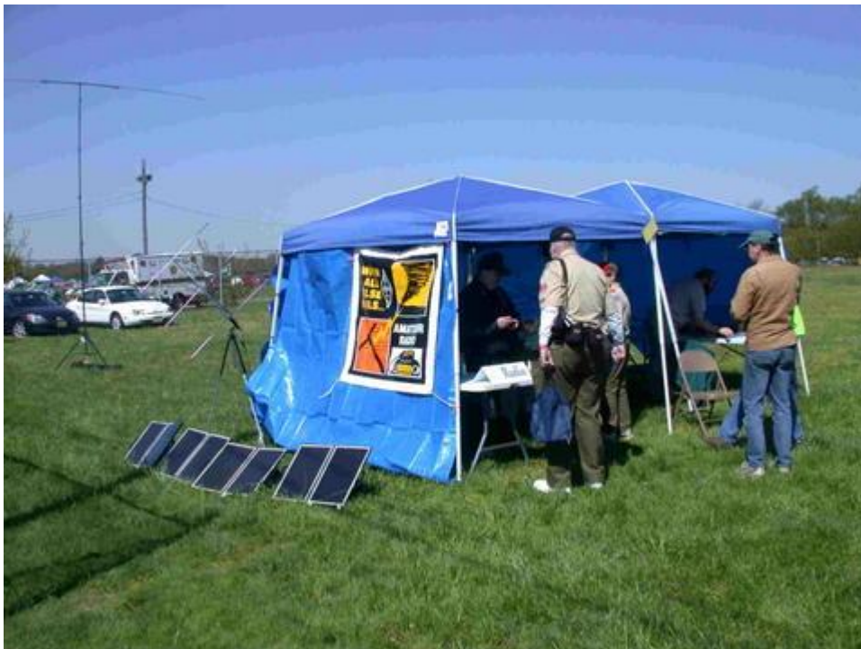
Solar-powered Amateur Radio Station in tents. Note the portable VHF/UHF satellite and HF antennas in the background
