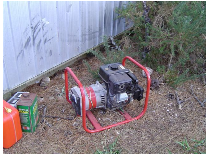
Roy's portable generator for AC power
