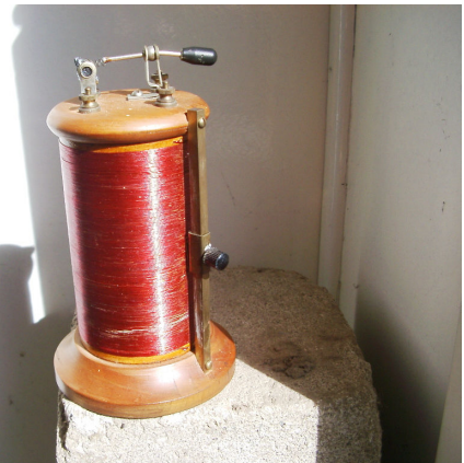
Pictured above is a Cats-Whisker set owned by Ian ZL1RCA. This set was constructed quite recently. The parts are all salvaged from something else. The frame was nicely turned from Rimu. The Station are found by moving the brass slide up or down the coil after adjusting the Cats-whisker on the top. It worked well after a good spot on the cats-whisker was found but selectivity suffered.
