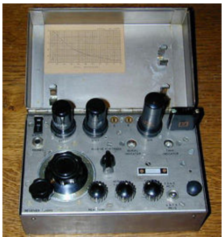
Paraset Radio, a self contained miniature transceiver supplied during WWII to Resistance forces. [Antonio Fucci Fano photo]
