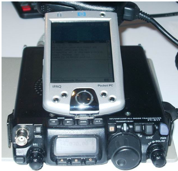
The PDA sitting on top of the FT817. 14.070 is a good frequency to receive PSK31
