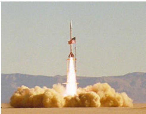
This 2002 CSXT attempt to reach space failed when the rocket engine exploded three seconds into the flight.
