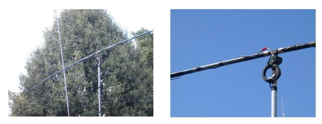
Another natty idea is two telescoping fishing rods with wire wound around instead of the usual fishing line. This set-up can be erected in seconds by expanding the fishing rods and then slipping into a 'T' piece on the top of a pole. The antenna can be rotated or held at any angle for the best reception. Plugs and sockets along the wire dipoles allow for operation on more than one band.
