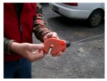
The two dipole sides are wound into two plastic plumb-bob cases. Harry uses Teflon coated wire and has marks at 10, 15, 20, 40, and 80 metre bands on the wire. He simply unwinds the right amount for each band.
