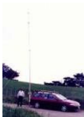
HF antenna mounted on the rear of the car
