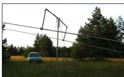
Sl. 71. Portabl EME antenski sistem YT1VP (2xEF 0213 by YU7EF)
