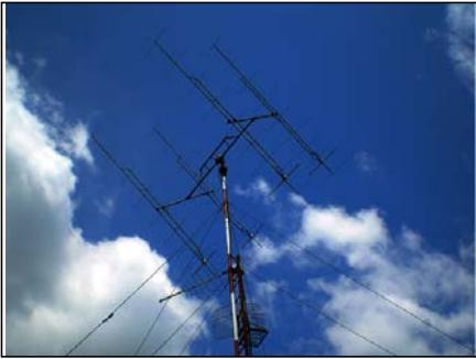
Sl. 66. Novi antenski sistem YT3I, 4x10el Yagi (EF-0210 by YU7EF)
