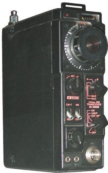
Sl. 68 Popularni prenosni SSB/CW transiver za 2m firme ICOM, model IC-202
