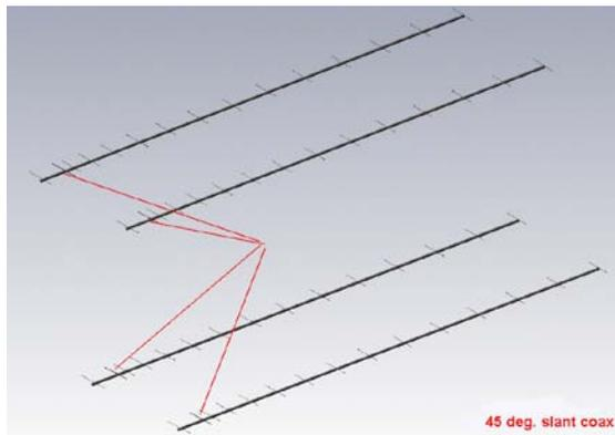
*Fig. 2 Yagi system with 45 deg slant coax cable*
