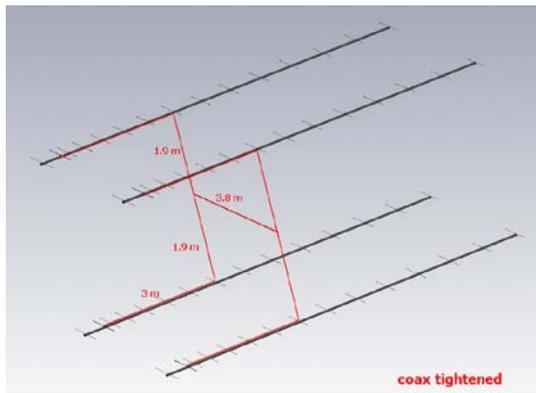
*Fig. 1 Yagi system with tightened coax cable*
