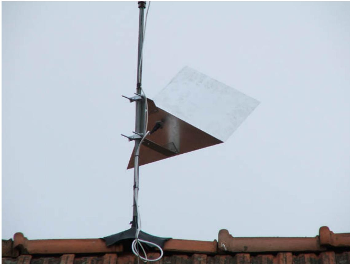
*Fig. 33. Shortened 3D corner reflector antenna built by 4N7TA*
