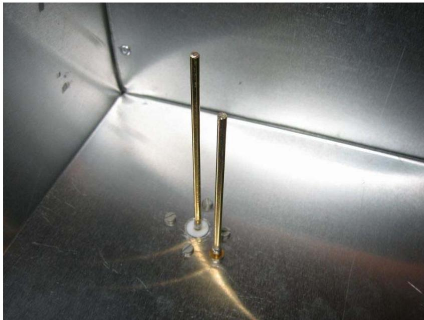
*Fig. 33. Shortened 3D corner reflector antenna built by 9A4QV*
