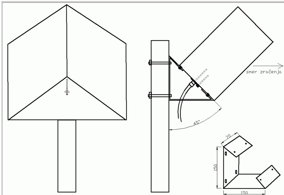
*Fig. 32. Proper mounting and radiation direction of antenna.*
