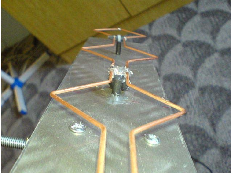
Feeding coaxial cable and BalUn position with polyethylene water protection of cables and soldered junctions
