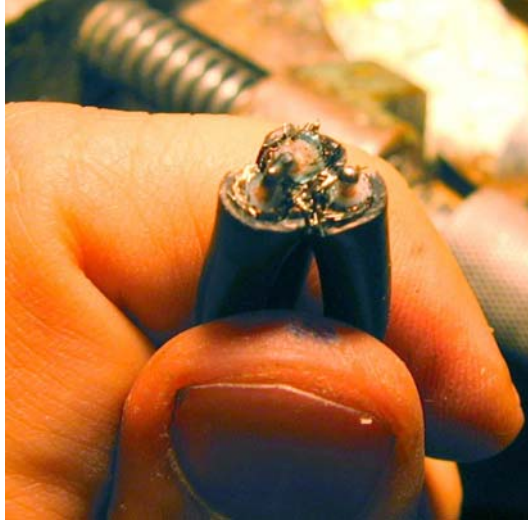
Preparation and soldering of half wave BalUn and feeding coaxial cable
