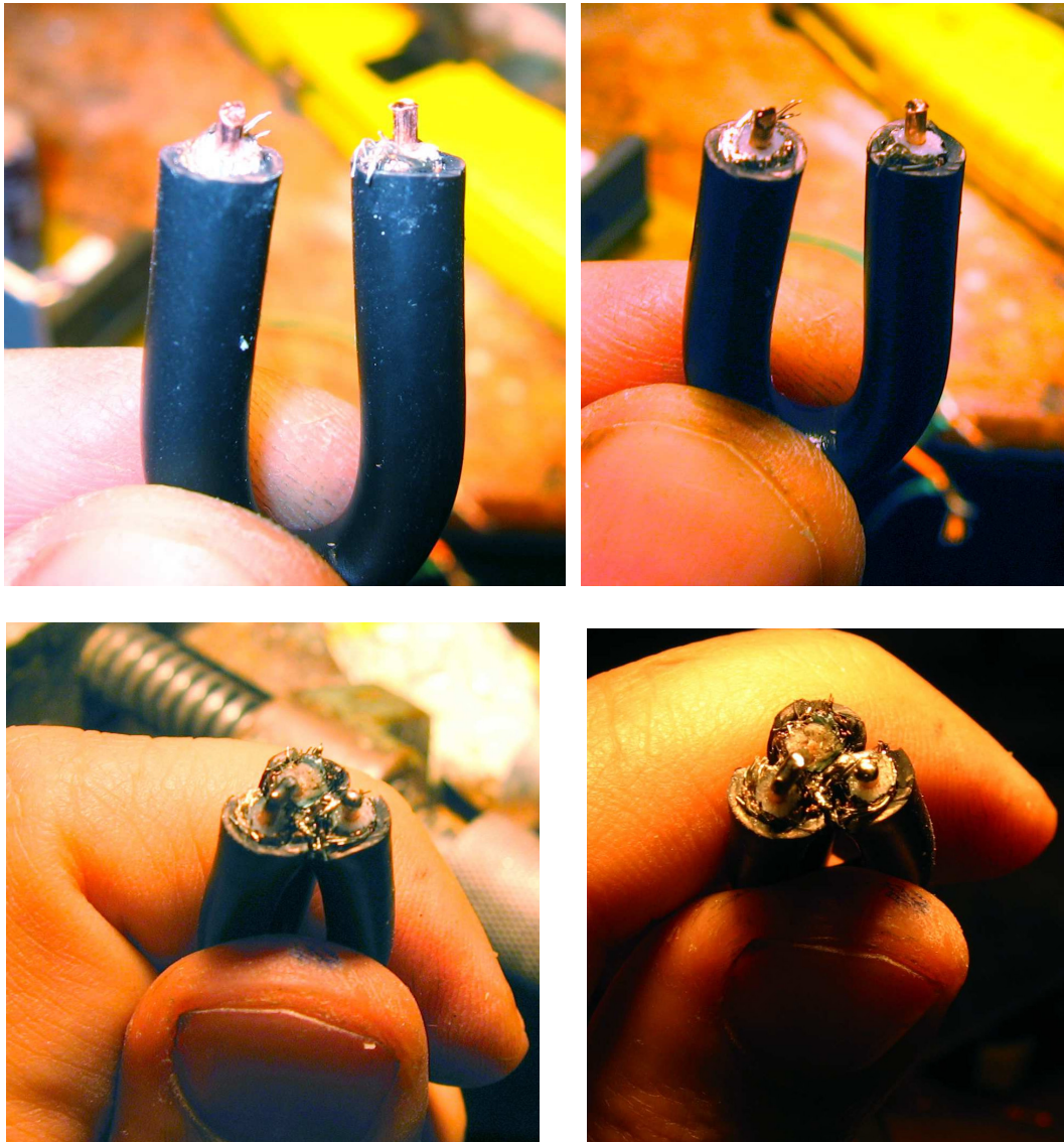
Preparation and soldering of halfwave balun and coaxial cable
