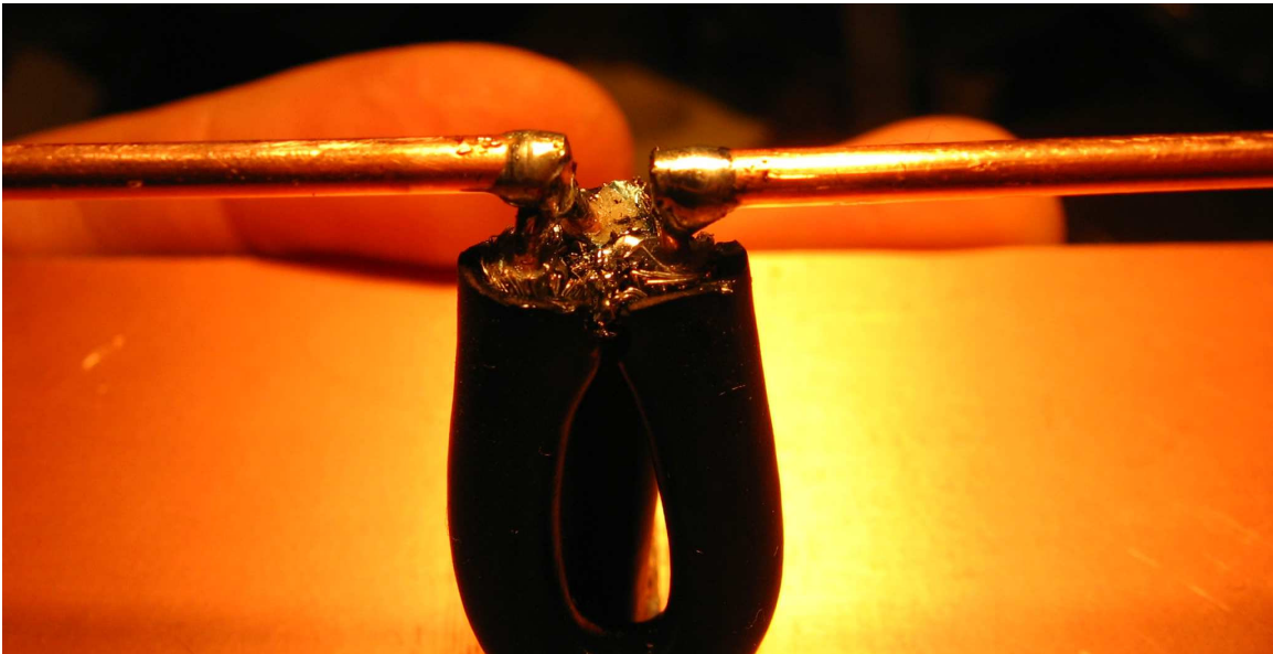
Balun and feeder soldered to radiation dipole
