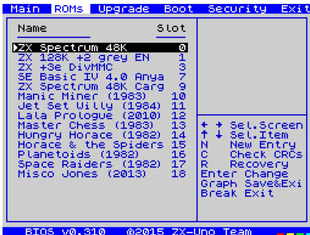
The Boot ROM can be chosen by pressing ESC (break) when the ZX-Uno shows its loading screen, this will affect just that boot. If you want to change boot ROM permanently you will need to enter the BIOS, go to the ROMs menu, and press enter on the chosen one, then select “Set active”.
