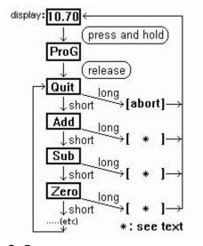
The program flow chart on the left shows how to enter programming mode, how to select a menu, and how to execute the associated function. To enter programming mode, press and hold the programming key (or connect pin 4 and
