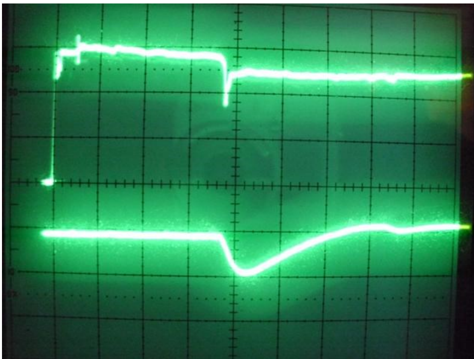
Figure 613 Beverage TDR traces - NorthEast
