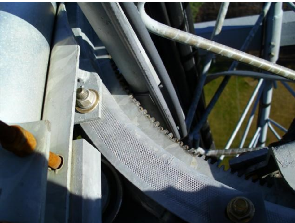
Figure 539 Damaged teeth on top ring.
