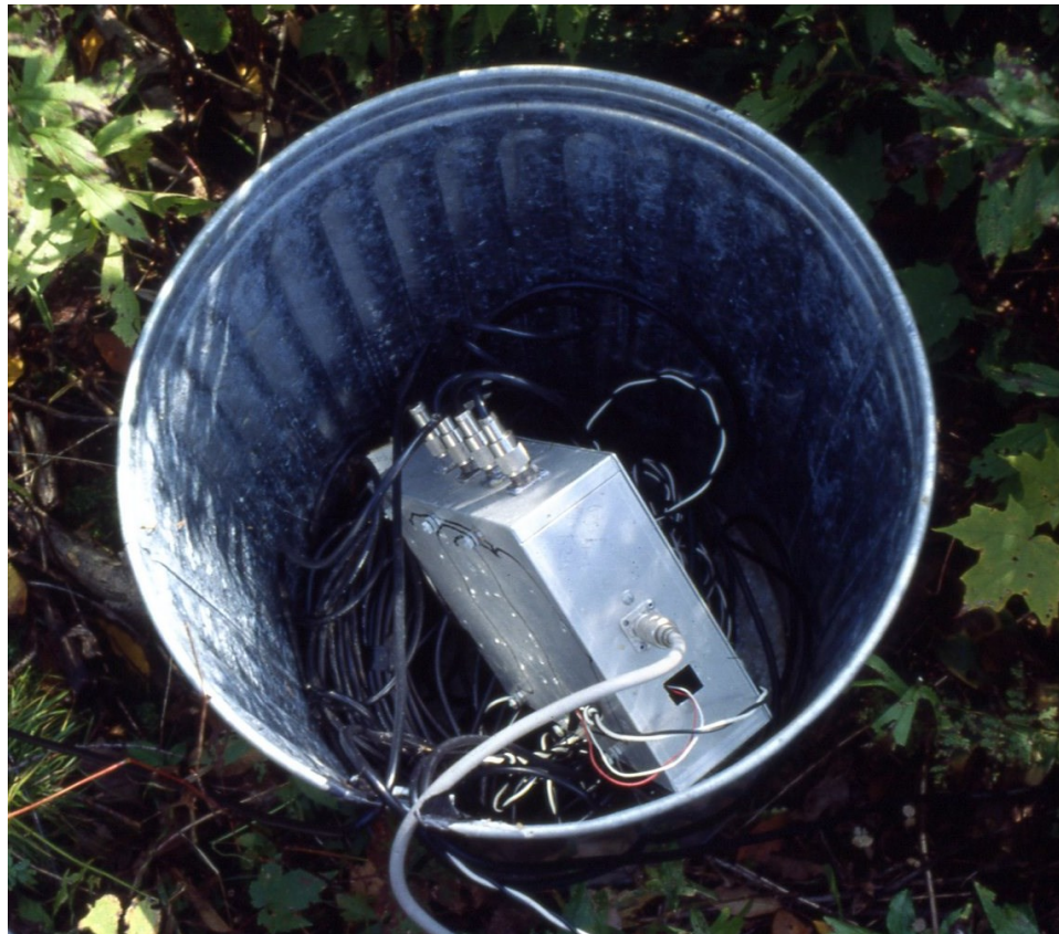
Figure 801 4-square phasing network in enclosure.
