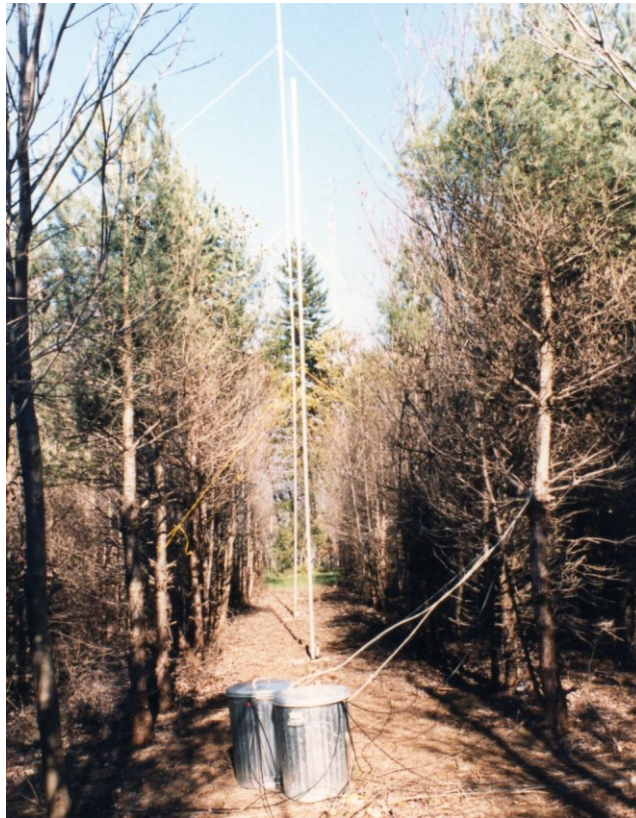
Figure 37 80m 4-square and 40m 4-square feed points and one set of verticals
