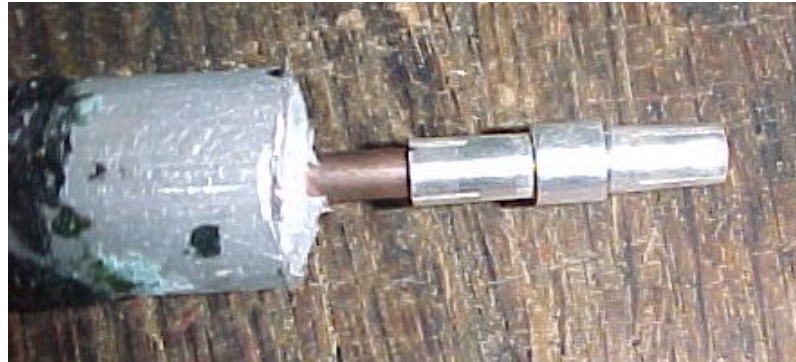
Figure 848 Center pin of barrel connector ready for shell
