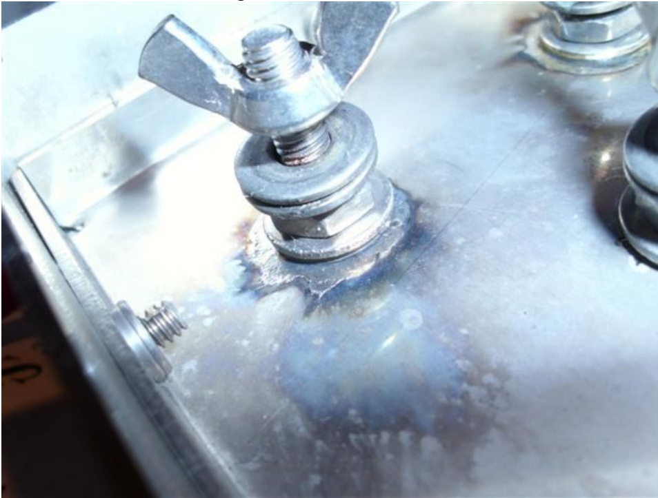
Figure 609 Lightning arc on outside of Beverage box
