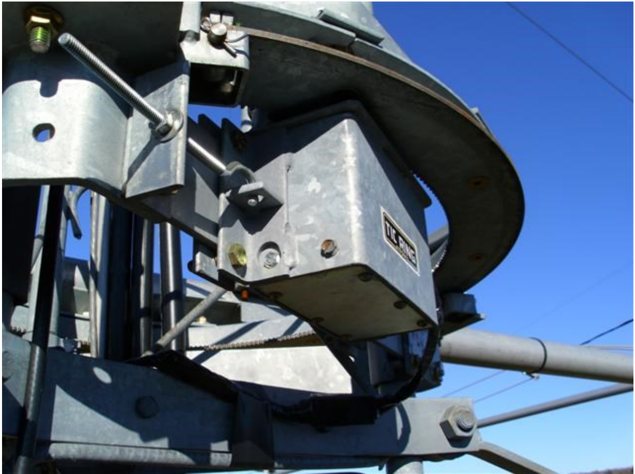
Figure 548 One of the lower ring motors, note they are fully enclosed now.
