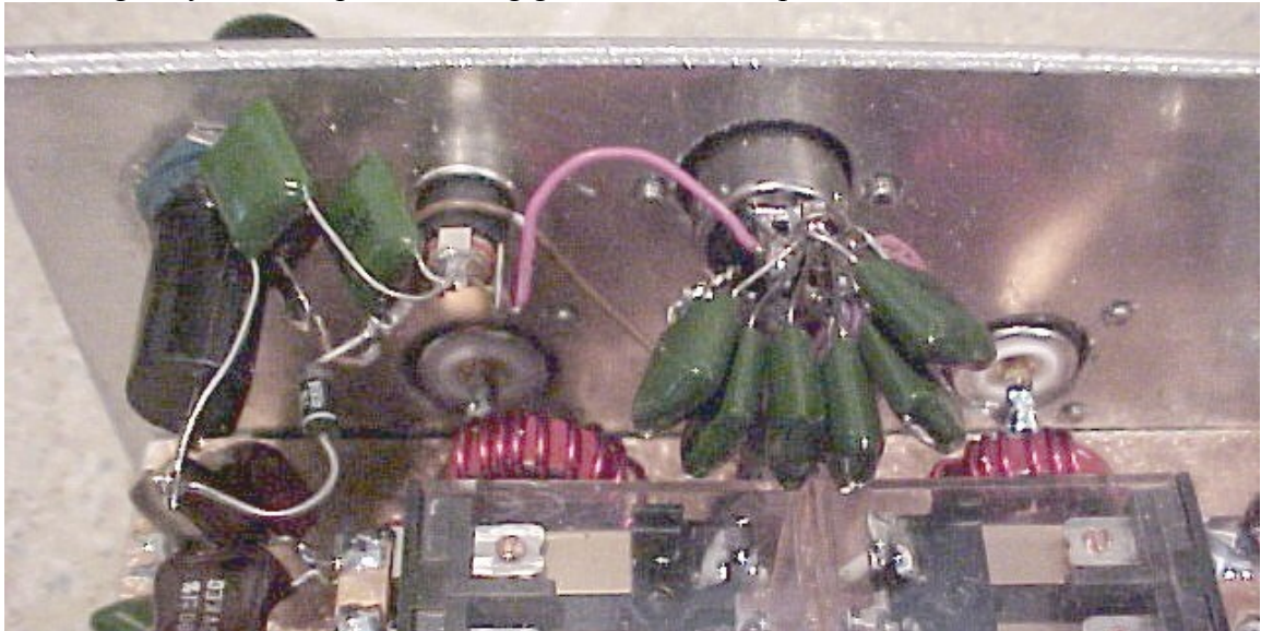
Figure 840 419A input line caps on control and power
