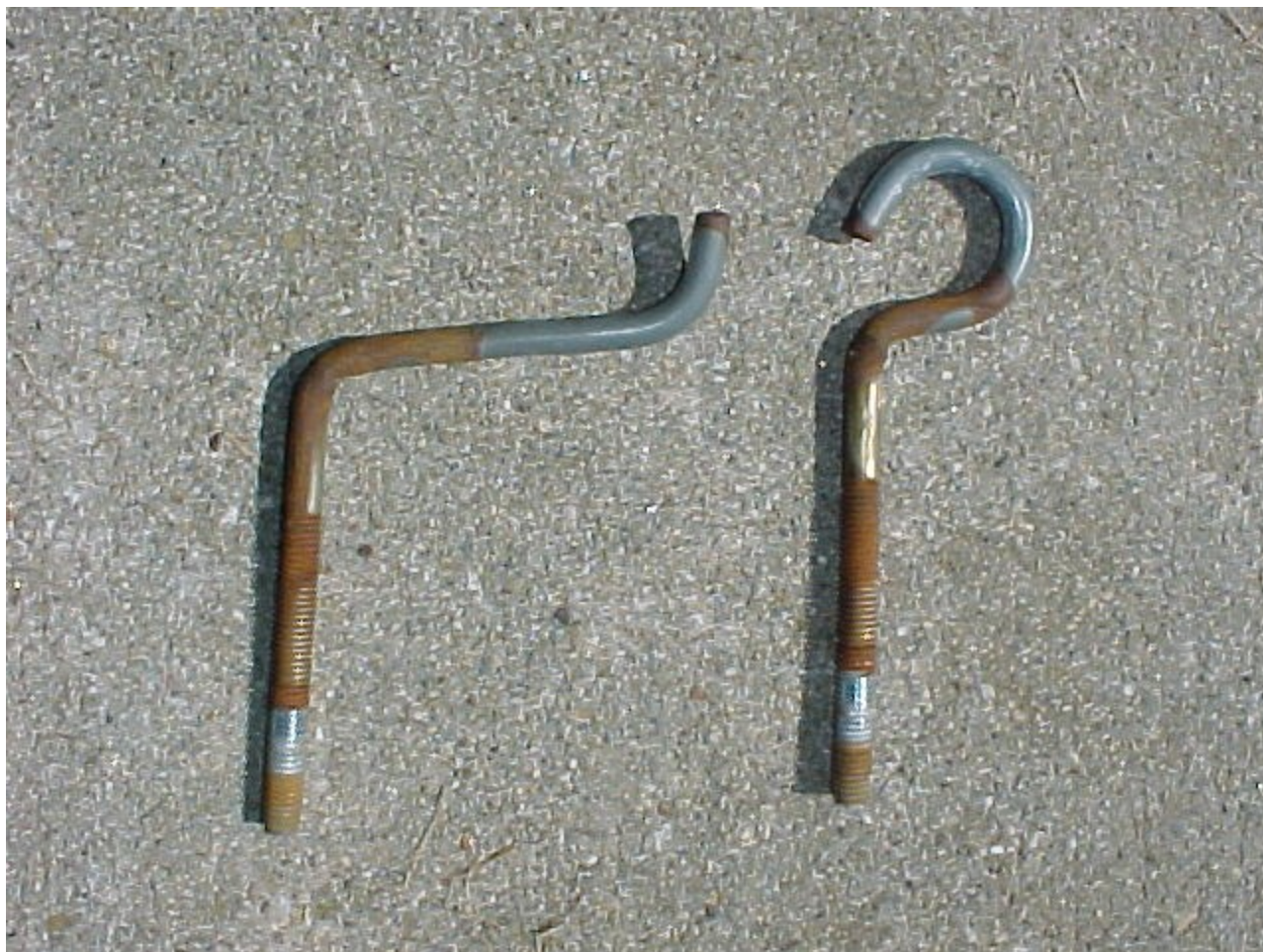
Figure 401 Those were the 3/8" eye bolts that held the boom truss for the lower 40m4l1dd... The one with the broken boom.
