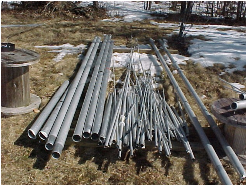
Figure 399 Pile of mostly bent bigger pieces, broken booms, and lots of element tips that may be at least partially salvagable.
