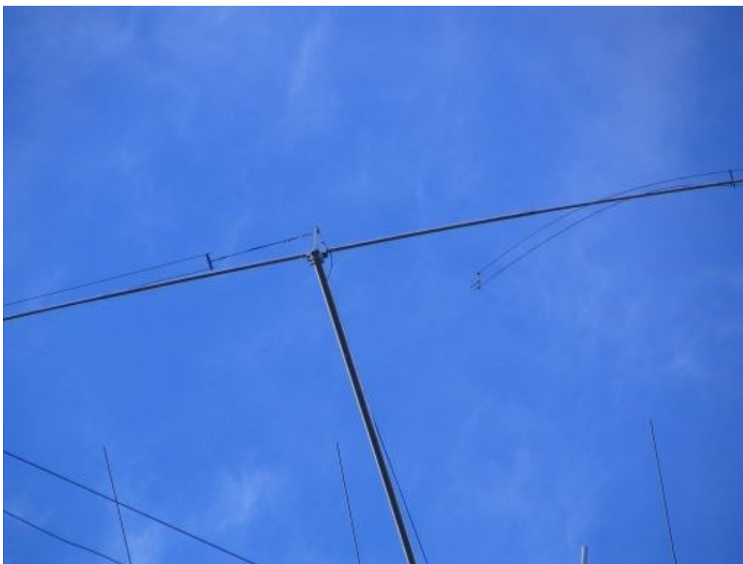
Figure 258 Broke 40M4LLDD element truss.
