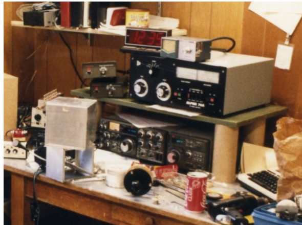
Figure 777 Cardboard tubes supporting amp shelf
