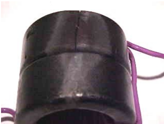
Figure 349 Overheated and cracked toroid.
