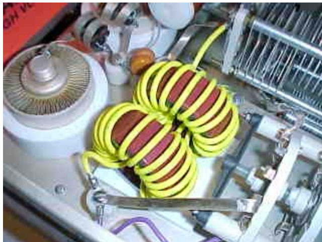
Figure 350 Two toroids in series with fresh cores and wire.
