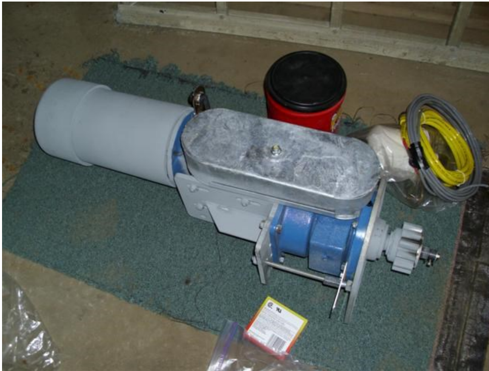
Figure 577 The motor and gear reduction unit.
