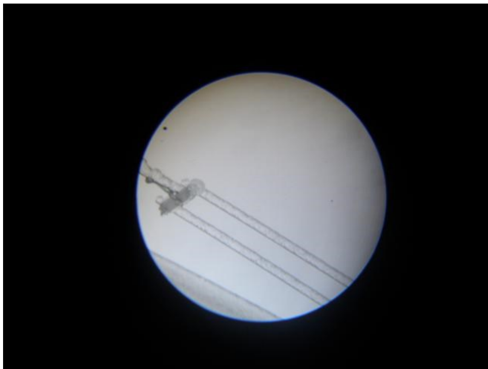
Figure 568 Ice on one of the 70' 40m4l1dd element loading lines.
