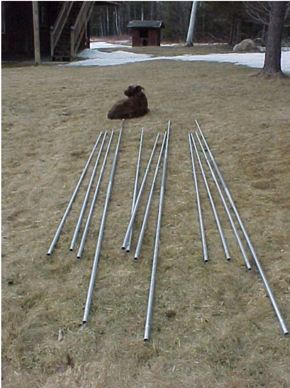
Figure 396 12 partially assembled elements with reinforcing in about 4 hours, including salvaging tubing from the scrap pile, cutting, fitting, and drilling.
