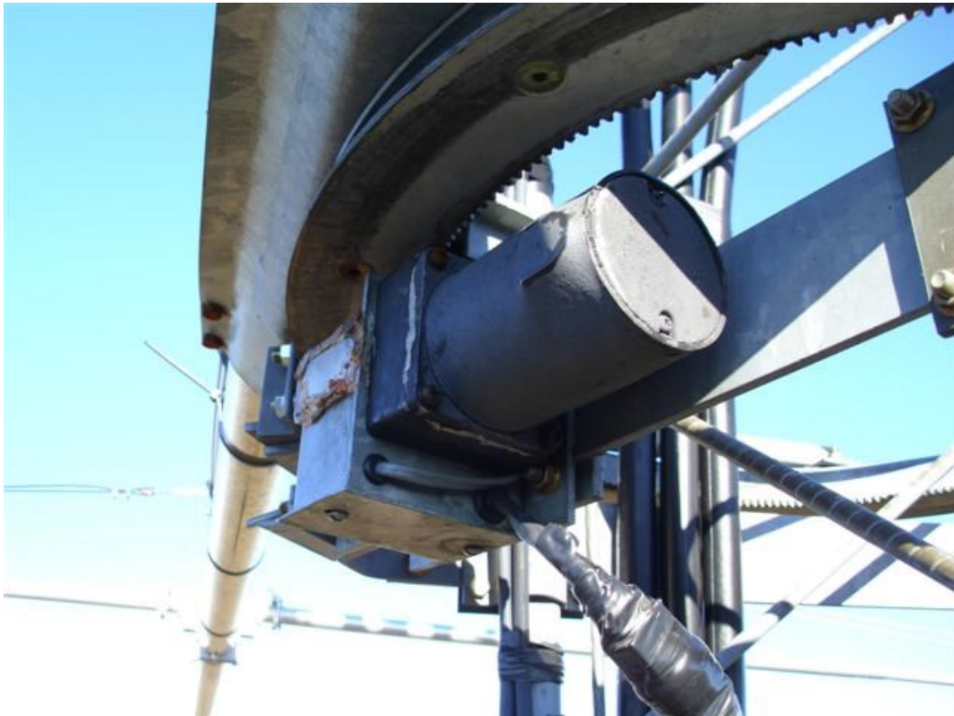
Figure 540 One of the top ring motors (note this is an older design.)
