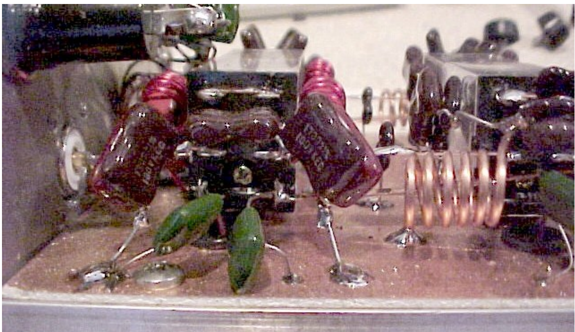
Figure 841 419A Two caps on each relay.
