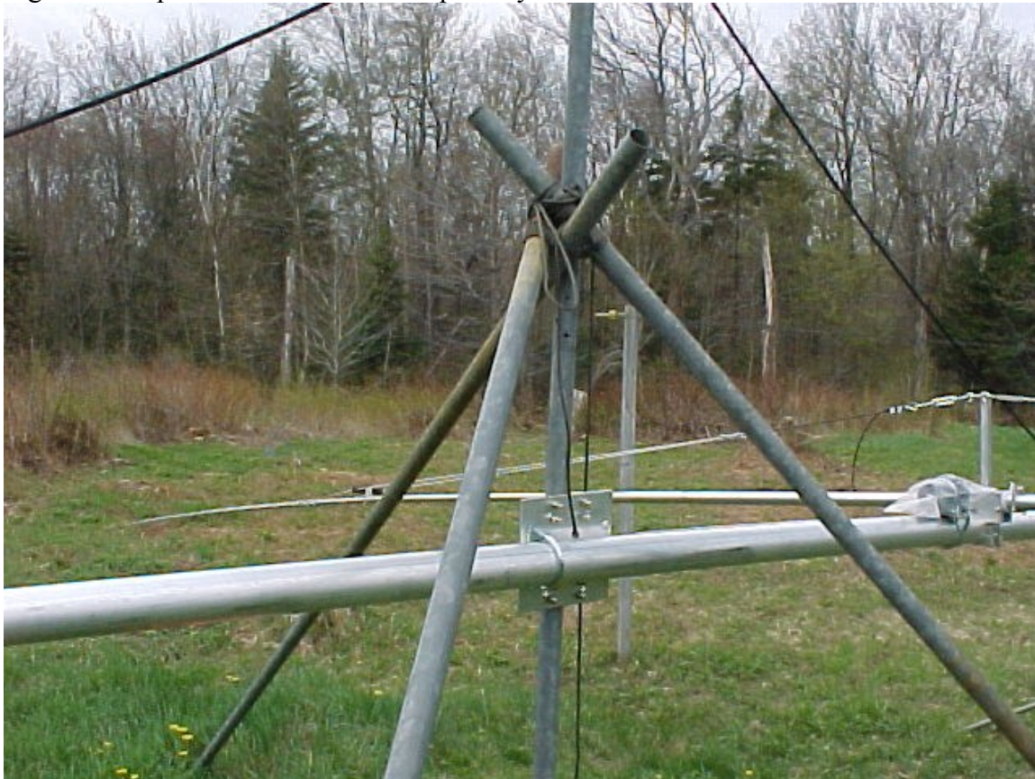
Figure 171 4 legged tripod for finding balance point.
