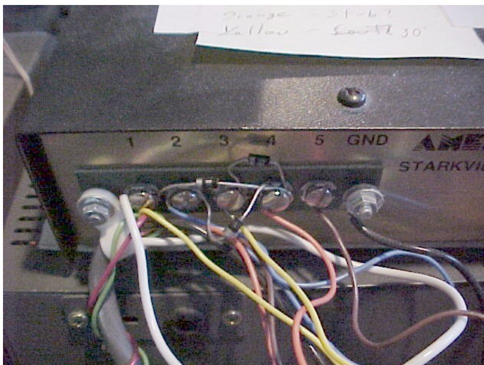
Figure 798 How the diode switching of the stack is really done for 10m/15m/20m
