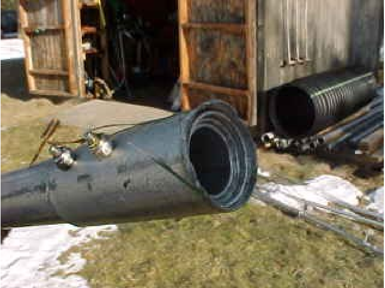
Figure 377 Broken swaged joint on 40M4LLDD-125
