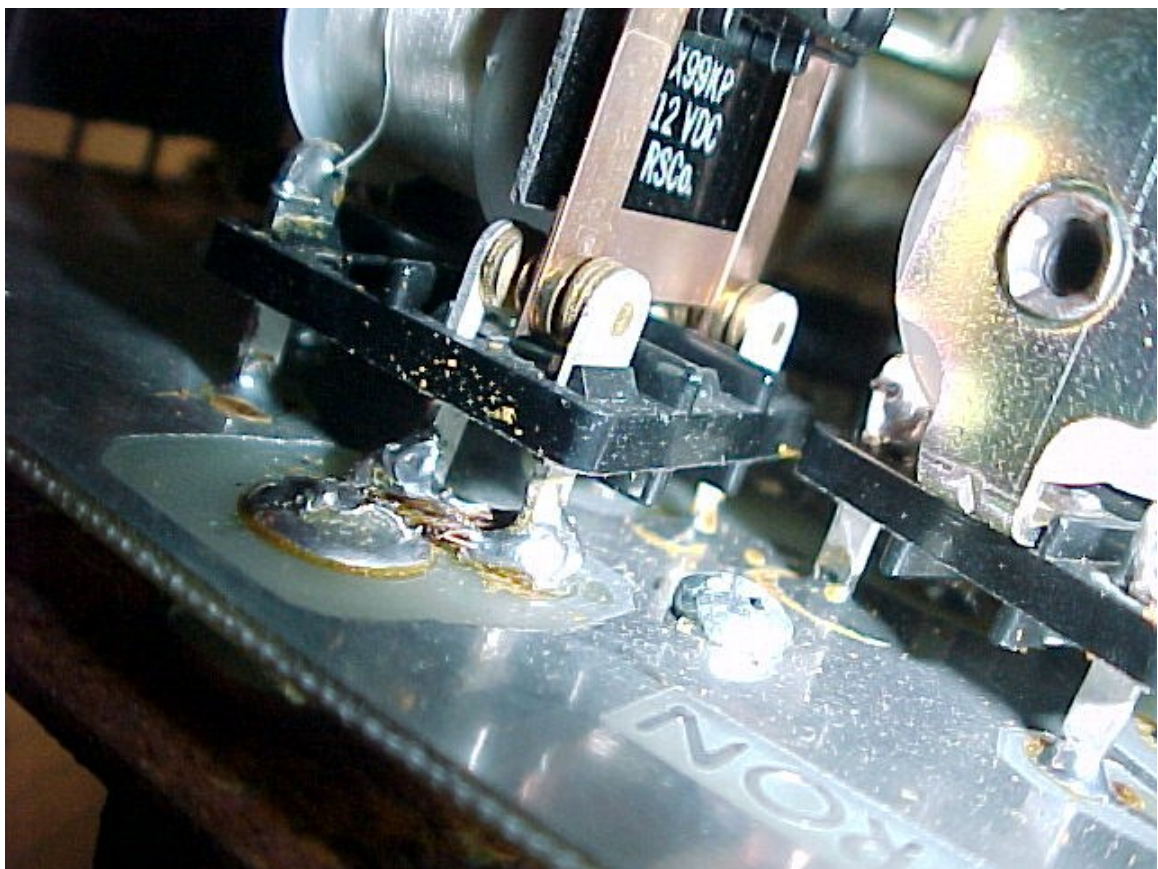
Figure 797 mod to ground RCS-8V output when not selected
