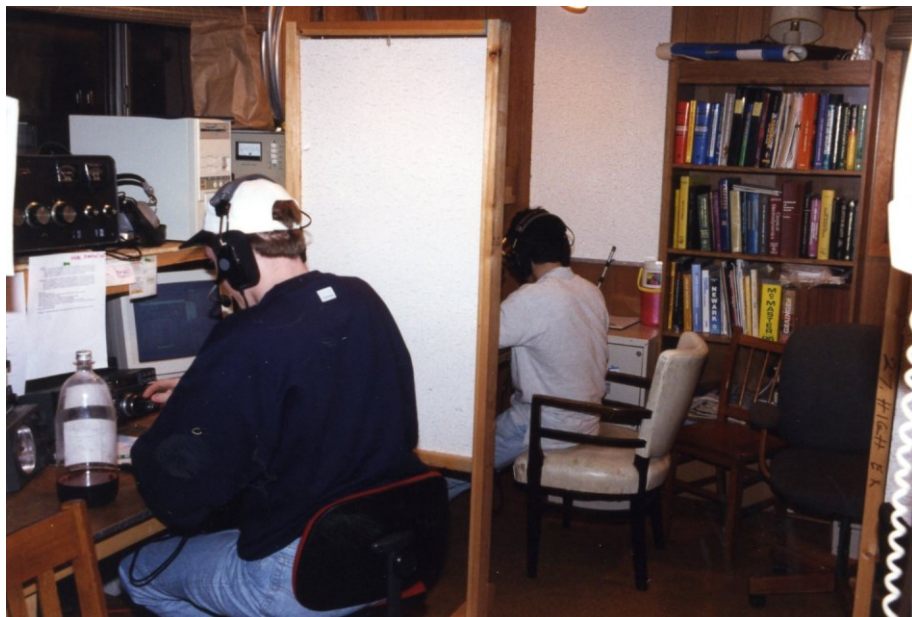
Figure 71 A sound damping partition between 20m and 40m.
