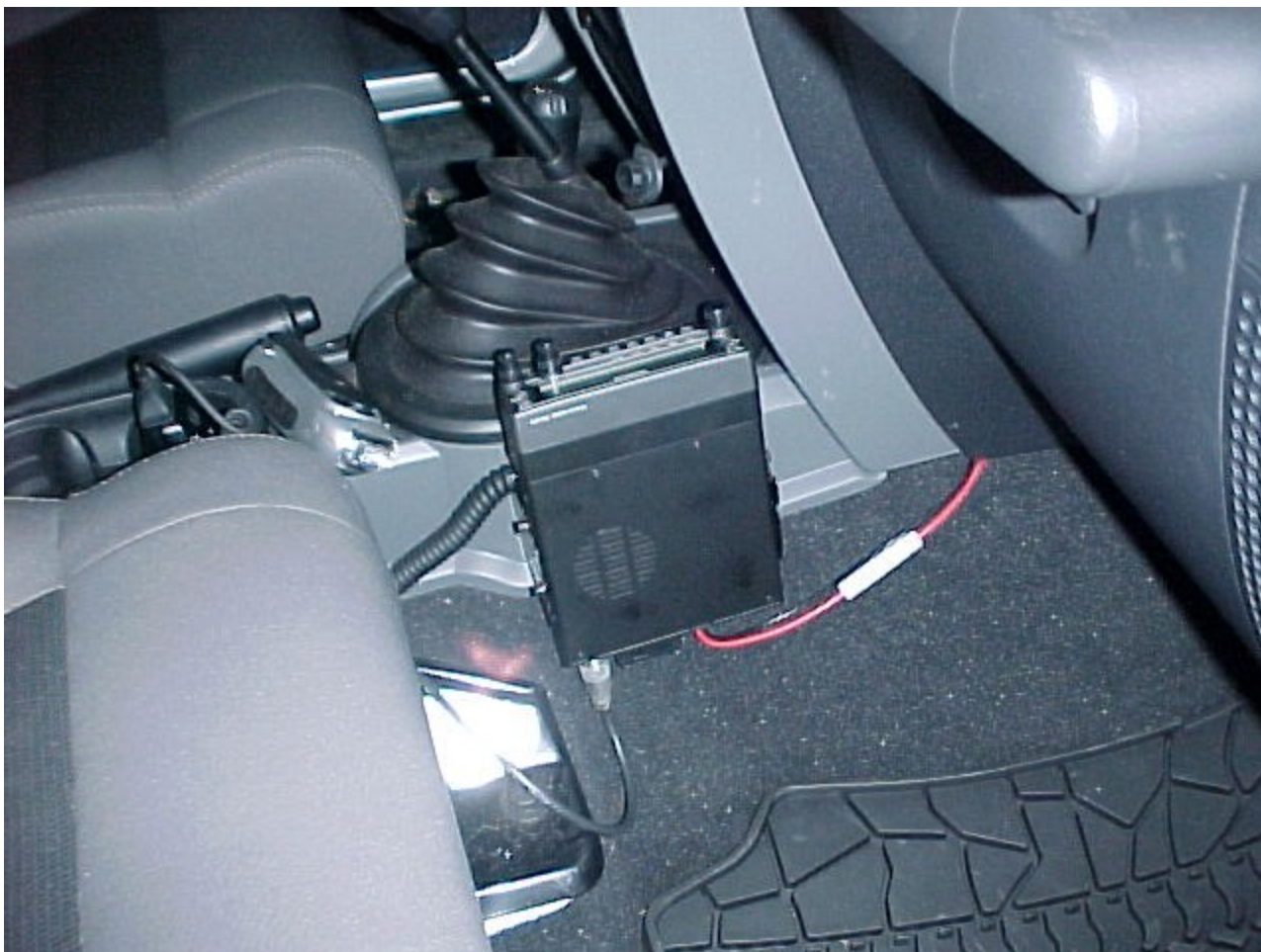
Figure 432 Inside VHF radio mounted
