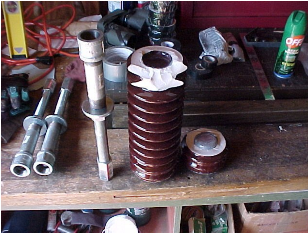
Figure 333 Broken insulator and tower jack.
