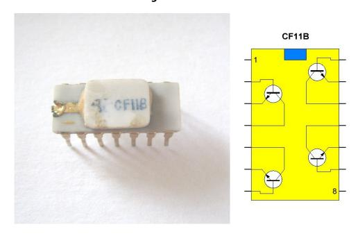
**REPLACED WITH 4 TRANSISTORS 2N2222 (***h*<sub>fe</sub> matched)
