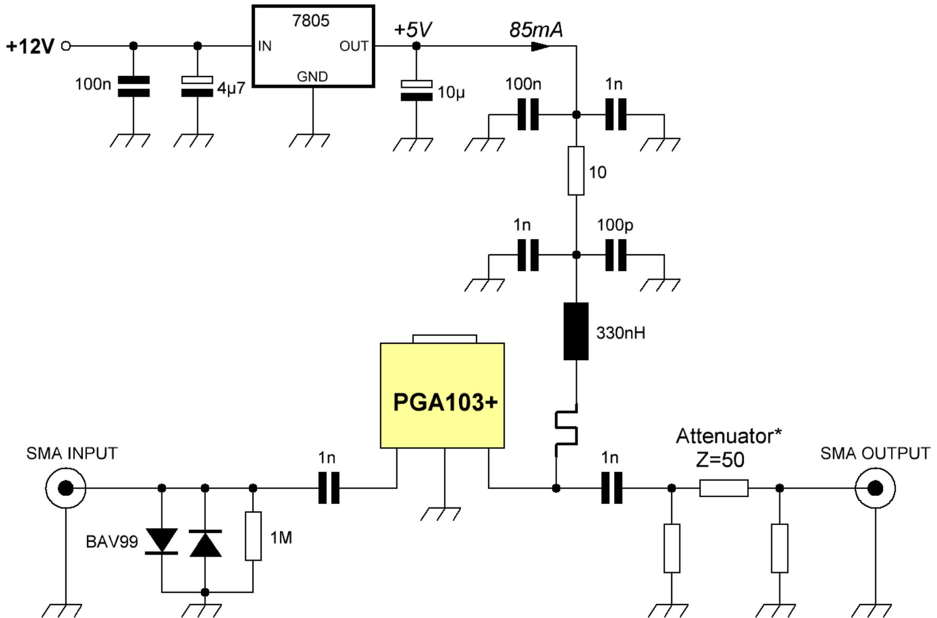
*Values of coupling capacitors and coil are not critical.*
