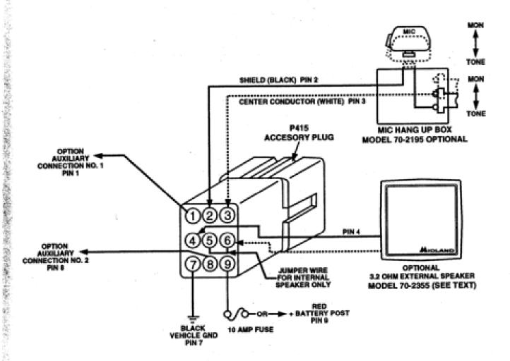
Figure 3 - 1 Under-Dash — Power/Accessory Plugs
