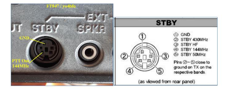
STBY connector *Mini DIN5 Male* is not used too often, but is almost same like Mini DIN6, has one more pin. Mini DIN6 was found many years between keyboard and PC, known as *PS2 connector*. I have a spare PS2 extension, so I can modify the cable for my purpose. Also you can use PS2 cable from an old keyboard.
