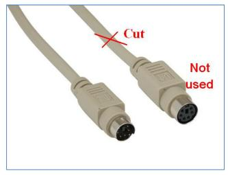
First step is to cut *Female* connector and and throw it away. GND pin and PTT Out can be identify using the ohmmeter. My cable has blue wire for GND and red wire for PTT 144MHz, but this isn't a rule.
