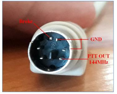
For better EMI immunity, connect shield wire to GND. My QROs are using RCA connector for PTT control.
