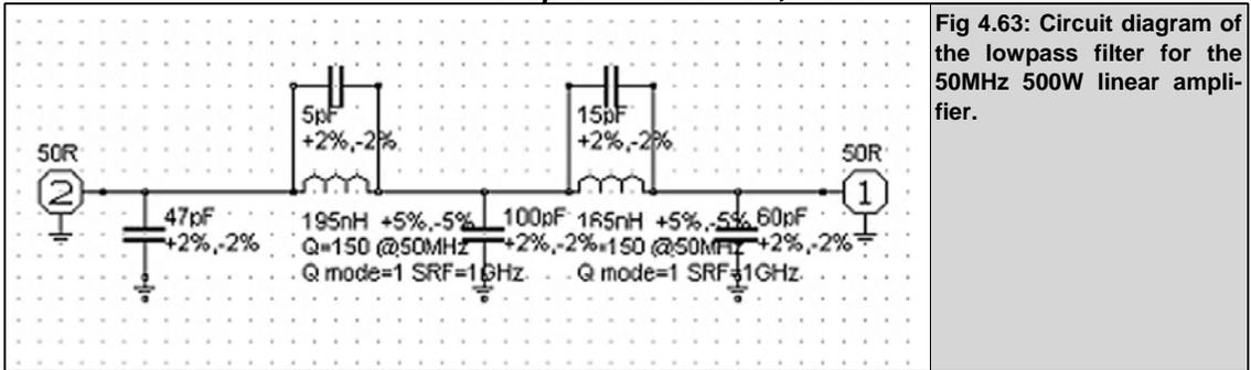
Fig 4.63: Circuit diagram of the lowpass filter for the 50MHz 500W linear amplifier.
