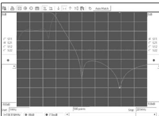
Fig 4.64: RFSim99 simulation of the lowpass filter for the 50MHz 500W linear amplifier.
