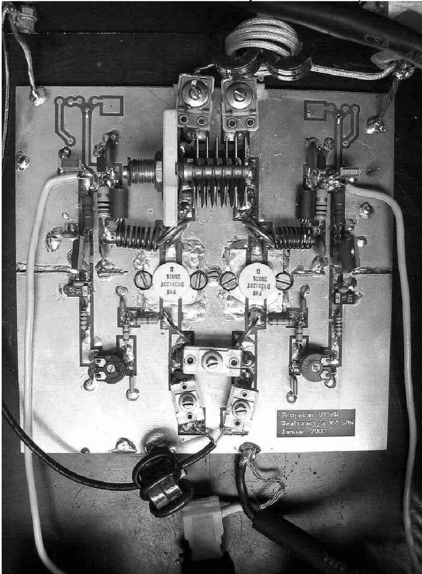
Fig 4.67: Picture of the assembled VMOS solid state 2m power amplifier.
