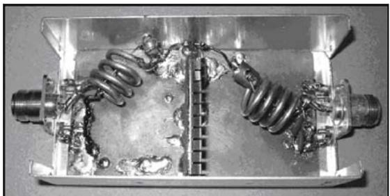
Fig 4.65: Picture of the lowpass filter for the 50MHz 500W linear amplifier.
