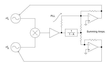
Figure 1: Bootstrapped PLL reduces oscillator instabilities.
