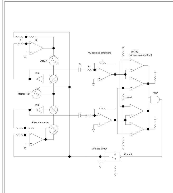
Figure 2: Bootstrapped reference oscillator moves slowly to a new frequency instead of jumping.
