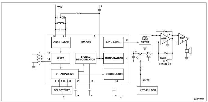
Figure 27. Remote Unit Receiver: 1.7MHz
