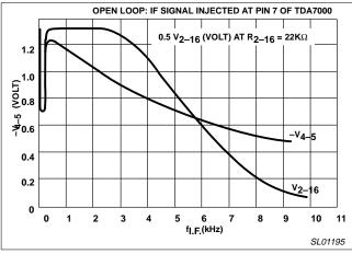
Figure 23. Demodulator Characteristics
