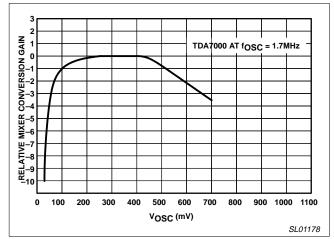
Figure 5. Relative Mixer Conversion Gain
