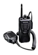
With its light yet strong aluminium die-cast chassis, the TK-3301 is built to survive hard knocks and drops. And thanks to its sealed case, it offers reliable performance in severe weather and environments. Even with the KMC-45 optional speaker microphone connected\* it satisfies or exceeds the stringent IP54/55 dust and water intrusion standards, as well as the US MIL-STD 810 C, D, E & F environmental standards.
