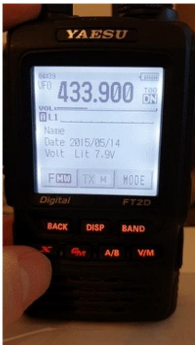
The openSPOT2 displays the currently active configuration profile number at the bottom right corner of the FT2D's display. Displayed information may look different on other type of C4FM/Fusion radios. The examples here are demonstrated using an FT2D.
