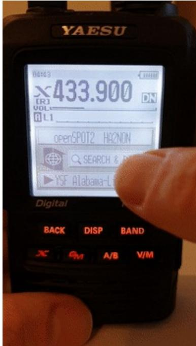
The first 5 entries will be your openSPOT2's configuration profiles. The list will contain the servers of the currently active connector. In case the currently active connector does not have a server list (ex. the Null connector), YSFReflector servers will be listed. To switch to an entry, select it using the dial and press PTT for a short time (or just tap on it in case you have a touch display).
