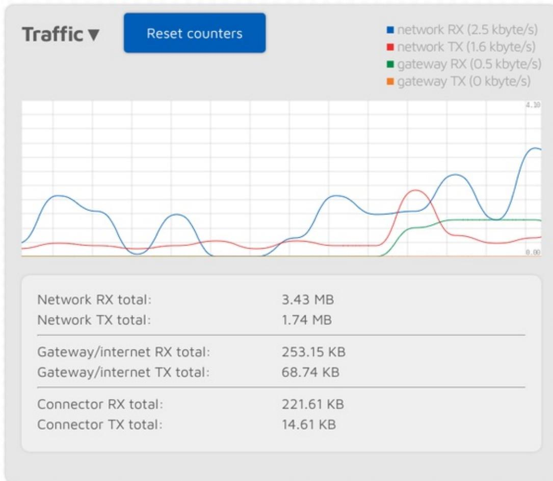
The **traffic graph** can be shown by clicking on the arrow at the top of the Traffic section. The **Network RX/TX total** shows total Wi-Fi traffic of the openSPOT2, the **Gateway/internet RX/TX total** shows the traffic coming/going from/to the gateway (which is usually the internet traffic consumed by the device), and the **Connector RX/TX total** shows the traffic used by the currently active connector.
