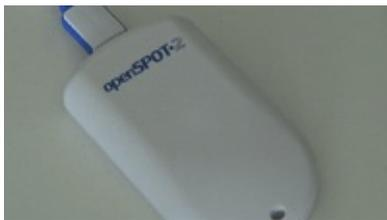
The AP mode is the openSPOT2's default mode of operation if no Wi-Fi networks are configured. AP mode lets you configure a Wi-Fi network which the openSPOT2 will connect in normal mode. You can switch between AP and normal mode anytime by pressing the [button](#) for 3 seconds.
