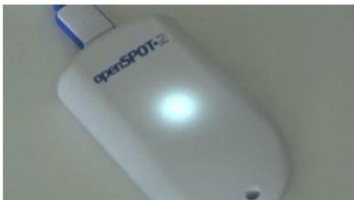
AP mode is the openSPOT2's default mode of operation if no Wi-Fi networks have been configured.
