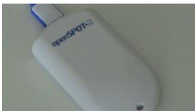
If the LED is pulsating like this, then the openSPOT2 is trying to connect to the selected server, but it can't for some reason. If it's not pulsating like on the animation, check the [LED states](#) section for more information about the current LED state.
