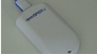
Enabling powersaving reduces the LED's brightness, turns off the [USB serial console](#) feature, and puts the Wi-Fi interface into power save mode. The built-in LLNMR and MDNS servers may not function properly in this mode, so opening the web interface by entering the openSPOT2's hostname into the browser (example: <http://openspot2.local>) may not work reliably. Use [SharkRF Link](#) to open the web interface.
