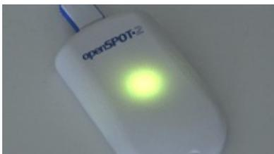
The LED will show this state only when the bootloader has been started manually.
