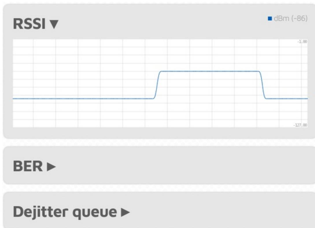
The **RSSI graph** shows receive signal strength from the modem. The **BER graph** shows received Bit Error Ratio during a call. BER is calculated also for packets received from the network, not just from the modem. The **dejitter queue graph** (only shown if Advanced mode is enabled) shows the number of packets waiting in the dejitter queue.
