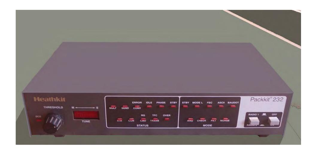
AEA introduces the PK-232MBX. The MBX has a PakMail "bulletin board" feature built into a daughter board, an upgraded PROM firmware, increased RAM memory, and a better battery memory backup arrangement.
