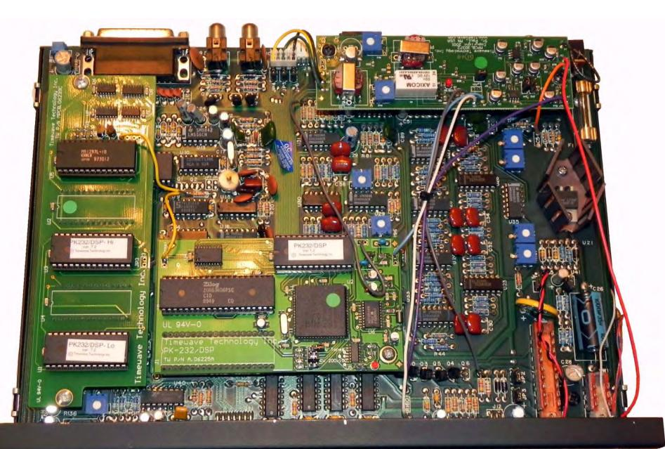
With the increased interest in sound card decoding for data modes, Timewave designs and sells an upgrade board to allow passing receiver audio through the controller directly to a computer sound card. The switching is done by software making it possible to work the hardware modes as well as software modes from the keyboard. Complete unit with sound card switching built in is the PK-232/PSK. List price is approximately \$550.
