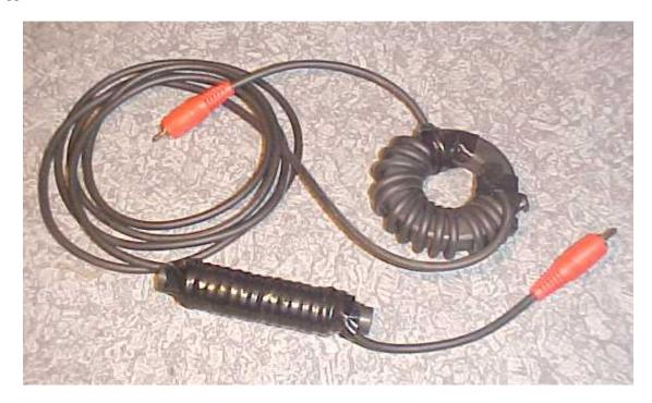
The cable shown above may be a little "over kill" but it might be necessary to put a ferrite device at each end of a cable to completely eliminate RFI. In most cases, I have found that one toroid or rod will work. Placement of the toroid or rod may be important as well, but not always. For instance, on keyboard cables, I like to put use a rod instead of a toroid and I place it near the input to the computer.
