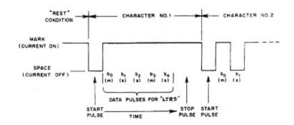
As you can see, the LTRS character is one Space stop bit followed by timing for 5 Mark data bits and 2 Mark stop bits. Now go back and read Chen's dissertation again on the advantages of using diddles and it should make much more sense now. Always use diddles when transmitting RTTY. Click <u>here</u> to hear what LTRS diddles sound like.
