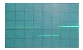
If you don't see a waveform or any change in state on your DC voltmeter, then your interface is not working. There is a very remote chance that your serial COM port is not working, but that is rare. You could change COM ports to see if the problem still exists, but odds are your interface is not correct.
