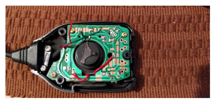
Step1: Unscrew the back from the microphone and carefully remove the back, paying close attention to how the PTT button on the mic is oriented and set into the slot, along with the orientation of the rubber button grommet. At the final modification step, the PTT button and the case have to line up without forcing and everything has to be reassembled exactly as it was when you opened it up.
