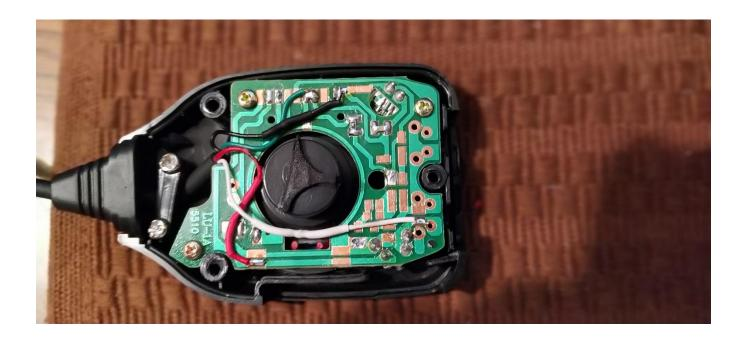
Step 6: The extended red wire, should be trimmed to an appropriate length to reach over and connect to the place where the white wire was before. See photo.
