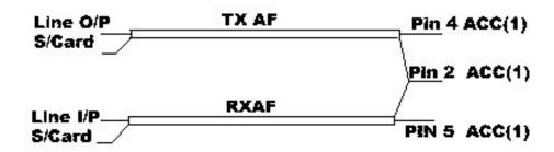
Audio connections for soundcard to IC746 Use miniature screened mic cable with mono 3.5mm mono jack plugs on soundcard ends.
