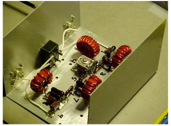
Toroid version of prototype of the "The AM BrickWall".
