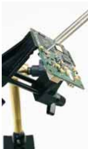
Touch up or rework QFP's and PLCC's with a small SMT soldering tip
