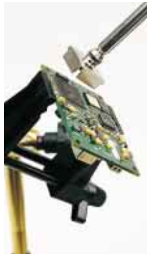
Rework QFP's and PLCC's using a CROWN tip on the high performance tool
