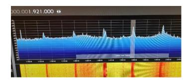
That in itself is an indication that the noise is manmade and probably coming from a switch mode power supply. Now the fun part. I turned each breaker off one by one and noted on some paper what I turned off and what the noise level was on the Icom as I had it on the whole time with the volume up.
