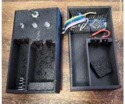
I designed and 3D printed the enclosure. The bottom half would hold the Arduino and the 9v battery that powers it and the top half would hold the LED's and power switch and provide the place for the batteries to be held while testing.
